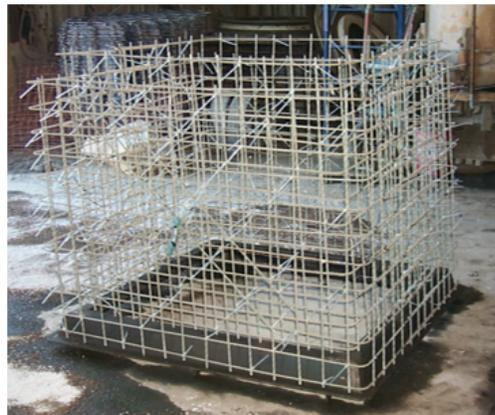
Fig. 2—A complete GFRP cage before concrete casting
