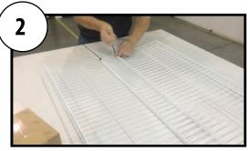
Secure both side of the grate using 4 zip ties. 2 zip ties per side.
