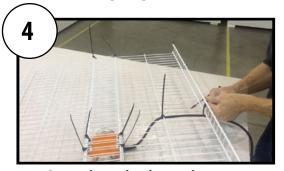
Secure the cord end using the zip ties IMPORTANT: Secure cord to the left side of upright angle of the grate.
