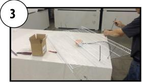
Remove the vibrator unit from the box and center it below the grate.
